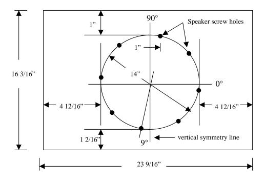
Off-set speaker screw holes, 1" or 9 degrees, from vertical symmetry line
