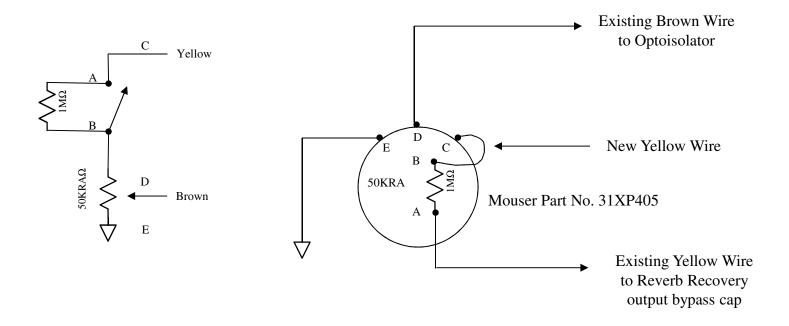
When pot is switched on, nodes A and B are shorted and thus the Intensity control works as usual. When pot is switched off, the normal 30% signal loss seen in the stock circuit is open-circuited, thus 30% more signal is seen at the phase splitter input. When turning the pot on and off, a pop will be heard unless a small amount of trickle current is allowed to flow between node A and B. Use a 1 Meg ohm resistor to eliminate the pop.
